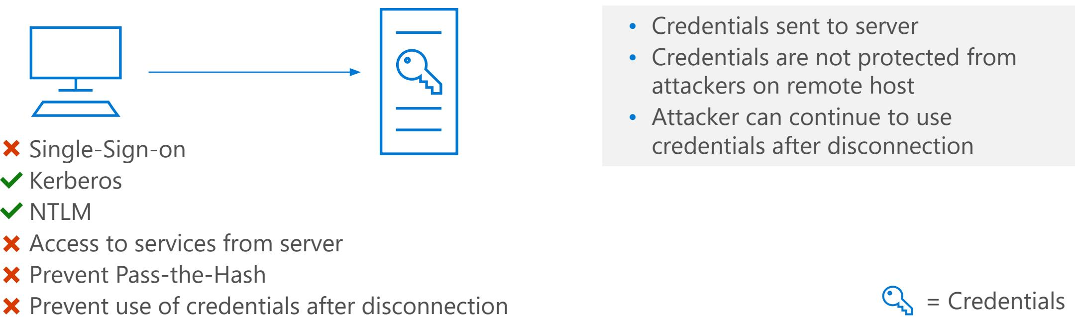
The following diagram helps you to understand how Windows Defender Remote Credential Guard works, what it helps to protect against, and compares it with the [Restricted Admin mode option](#):
